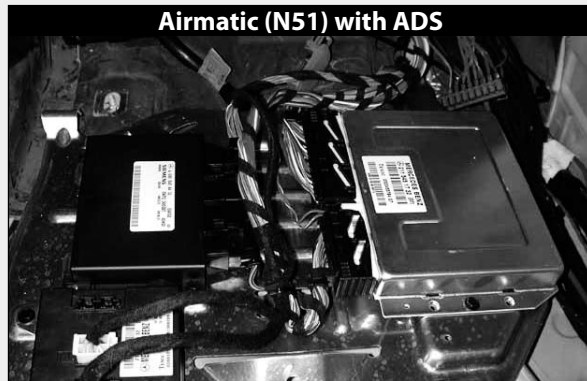
Unscrew 3 bolts holding the aluminum bracket
